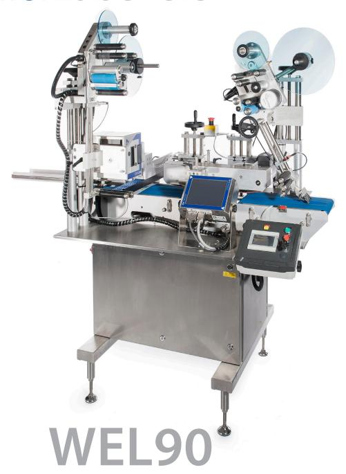
The Premier WEL90 (Wide Edge Leading 90) is a fully automatic labelling system designed for the meat and fish packing industry to enable multi-pack stacking and eye level shopping to encourage easy label reading.
